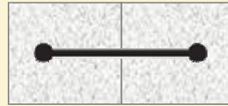
**Dumbbell Shapes** without center bulbs are suitable for construction or contraction joints where little or no movement will occur.
