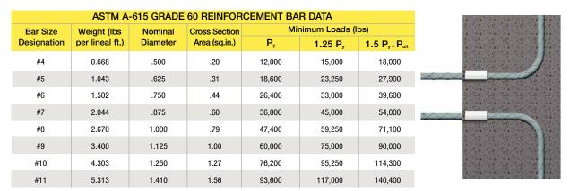
ACI 318 2005 Section (12.14.3.2) requires a full mechanical splice to develop at least 125% of the specified rebar yield strength (P<sub>w</sub>). Threaded Rebar Splice must have ultimate strength (P<sub>w</sub>) equal to or greater than 125% of the specified rebar yield strength (1.25 P<sub>y</sub>).
