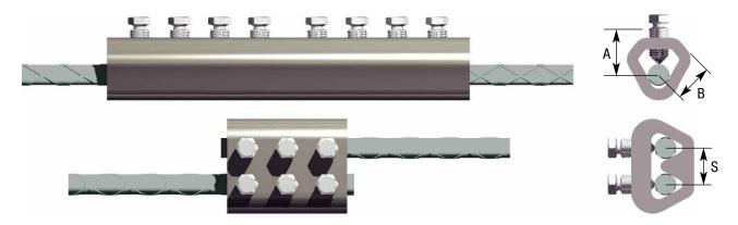
Tightening the lock-bolts generates a positive mechanical interlock as the rebar deformations are pressed into the ductile steel wedge-shaped body of the connector. Visual inspection is easily accomplished; just verify that the heads of the lock-bolts have sheared off during the tightening sequence.
