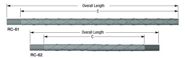
The RC-61, RC-63 and RC-64 Splice Bars are manufactured from Grade 60 deformed rebar material and are available in all of the corresponding sizes to the Threaded Rebar Coupler. After the Setting Bar has been placed and the concrete has set the Splice Bar is threaded into the Setting Bar to complete the splice. Splice Bars are available in the following configurations: RC-61 straight, RC-63 90° bend, RC-62 threaded at both ends and with a RC-64 return bend.
